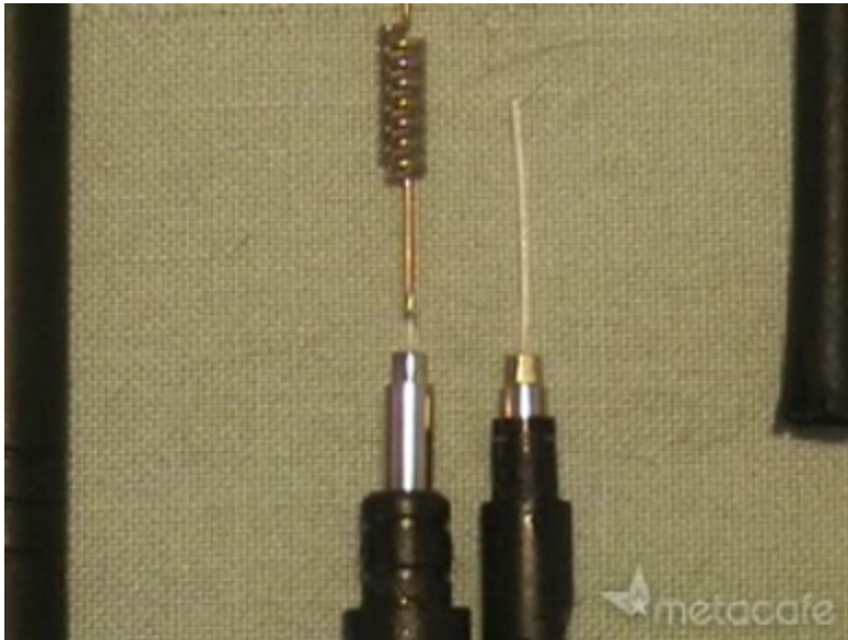
Figure 1 Video by babblin5.com showing how to turn a regular Wi-Fi antenna into a high-gain one
